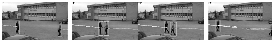
Fig. 3. Tracking results on our data set (frames 2555-2606). Two person moving toward to each other, turn around each other, then go back away. Thick and thin white lines separately represent their trajectories produced by tracking algorithm.
