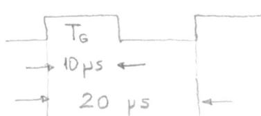
$$T = 2 \cdot T_G = 20 \mu s \Rightarrow f = \frac{1}{T} = 50 \text{ kHz}$$
