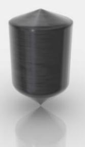
Mono-crystal Silicon Ingot scale: wafer level (~300mm / 12 inch)
