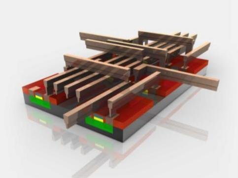
Metal Layers - scale: transistor level (six transistors combined ~500nm)
